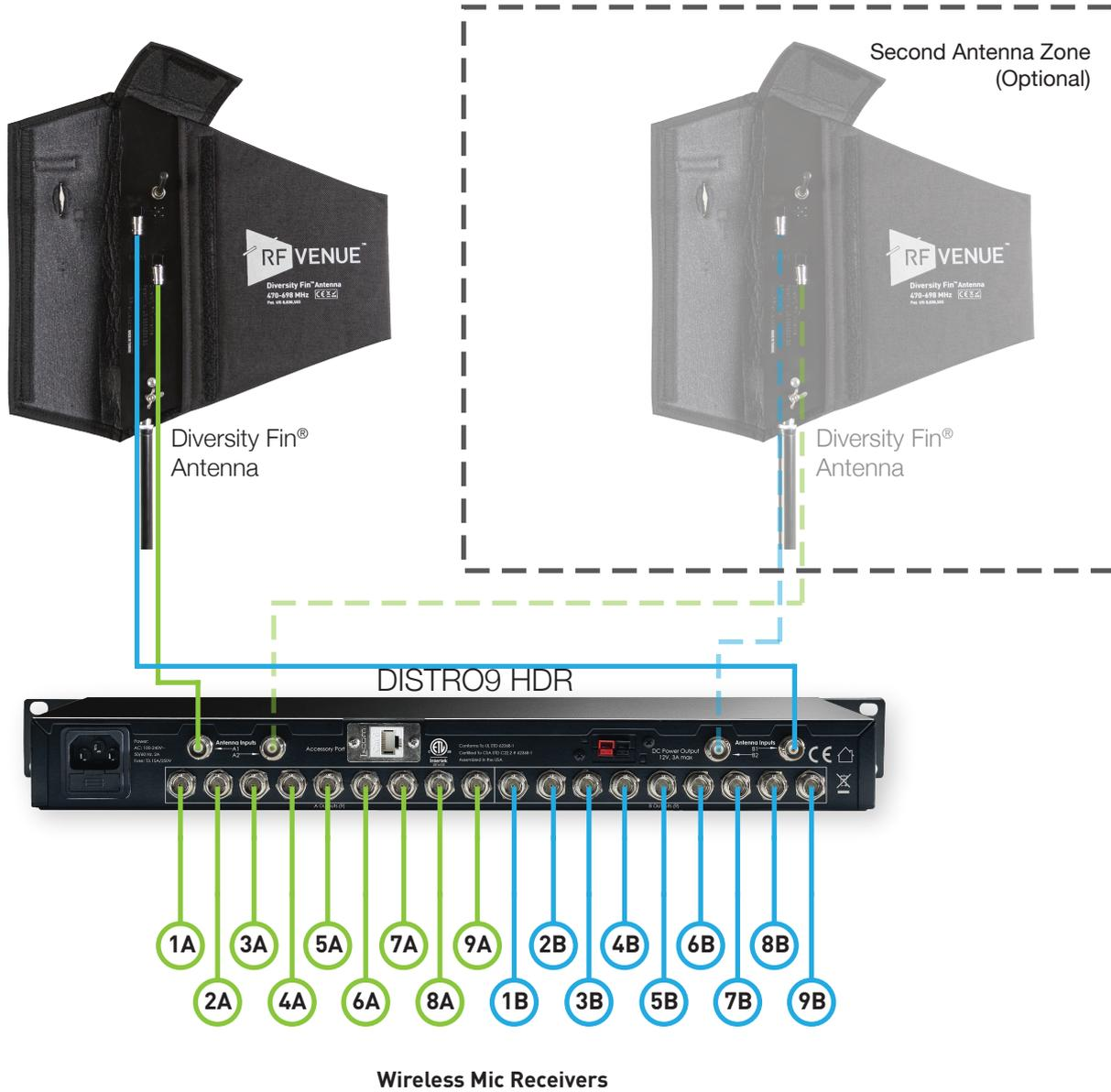
\*Note: All outputs are equivalent. Any "A" can be paired with any "B" and any pair can be cascaded.
